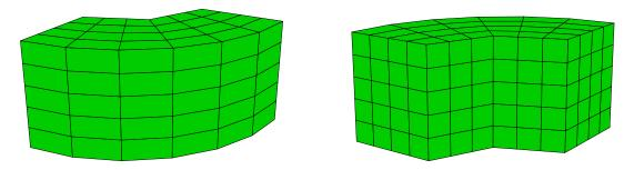
Figure 5.5: Three-dimensional Blended Mesh
