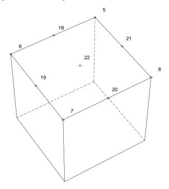
Figure A.4: Node Specification on 3D Master Block.
