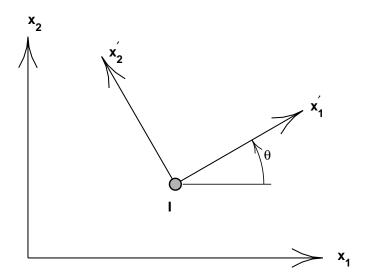
Figure A.6: Coordinate rotation for node I.
